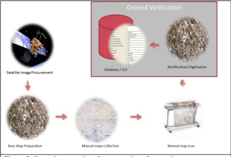
Figure 2: Step wise procedure for conversion of manual maps
