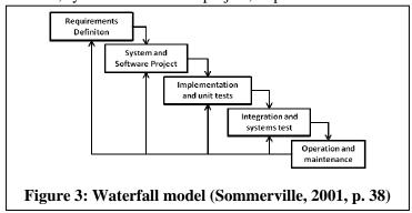
tion and system tests, operation and maintenance to the development of the software (Sommerville, 2001). In this process, the activities are developed in a sequential way and all the system requirements have to be defined by the client in the beginning of the project (Figure 3).
